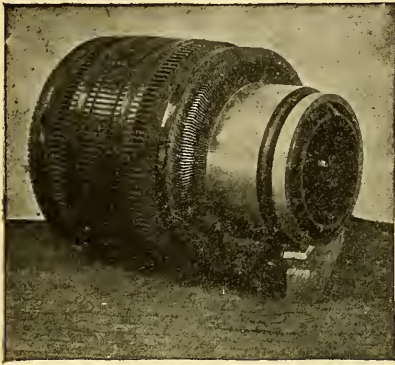
FIG. 201.—A completely finished armature ready to be fitted on its shaft; the windings are held tightly in place by the binding wires, several bands of which can be seen. Two ventilating ducts can be seen in the core.
